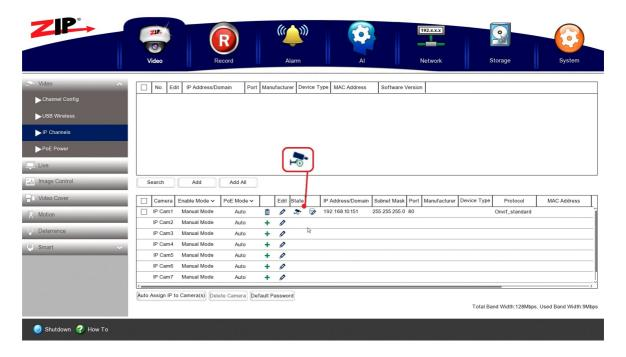
If the NVR can't connect to the camera then the symbol will be red.
